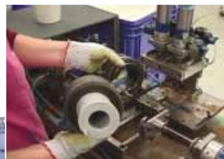
Former RTV production: Manual demoulding as well as casting and curing deflectors.
